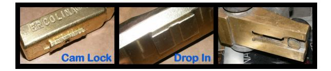
What do you do when you have counterbending dies with both versions of mounting? Simple, you contact your local dealer or sales representative and ask them to get the new **CBADP**, counterbending die adaptor plate. This high quality, machined, aluminum bracket enables users to quickly interchange between both mounting styles of counter bending dies.
